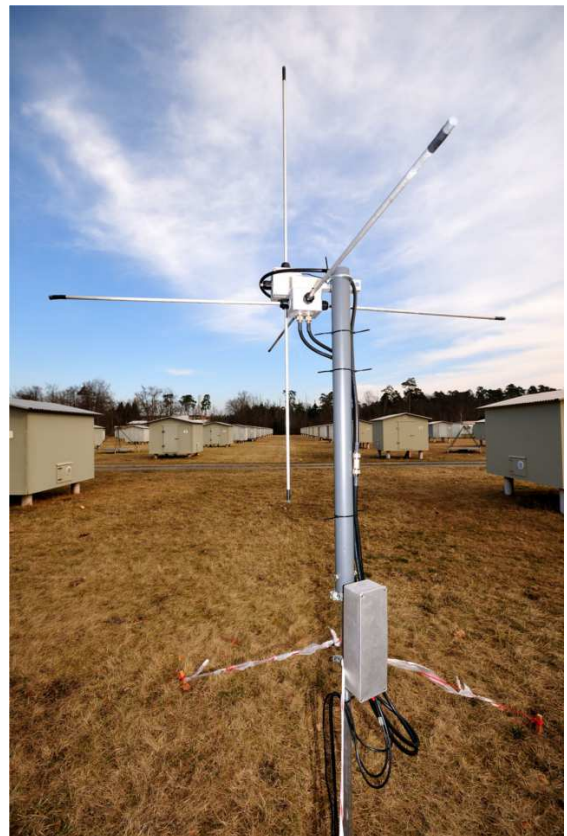
Figure 1: Photography of a tripole antenna station. The metal box at the pole is the housing of the pre-amplifiers.
