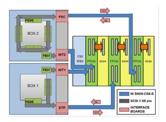
Figure 4: layout of the data acquisition system. The three FPGA are used to acquire monitor data
