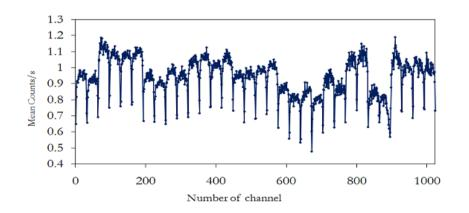
Figure 5: average number of counts per second for the 1024 channels of the pixel chamber.
