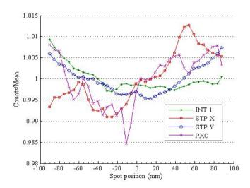
Figure 8: uniformity of the chambers as a function of the X position along the horizontal central line. The average number of counts in each point, normalized to the average over all the 37 points, is shown.
