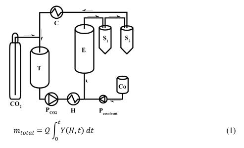
The kinetics of SFE extraction can be described through the Overall Extraction Curve (OEC) equation. The formula [Equation (1)] describes the relation between the extracted solute  $(m_{total})$  with the time of extraction and amount of flowed solvent, where Q is the flow rate of the supercritical fluid, Y(H, t) is the ratio of solute mass to solvent mass at a given time (t) at the extractor outlet (H).
