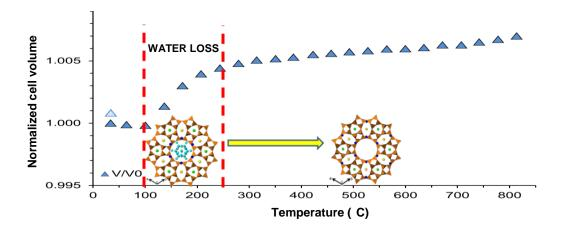
The high thermal stability of the synthetic zeolite K-L: dehydration mechanism by in-situ SR-XRPD experiments
