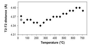
Table 1. Unit cell parameters of zeolite  $\boldsymbol{L}$  as a function of temperature.
