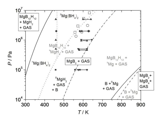
Figure 3. Calculated driving forces for the dehydrogenation of  $Mg(BH_4)_2$  into different products for  $P_{H2}=1$  bar.
