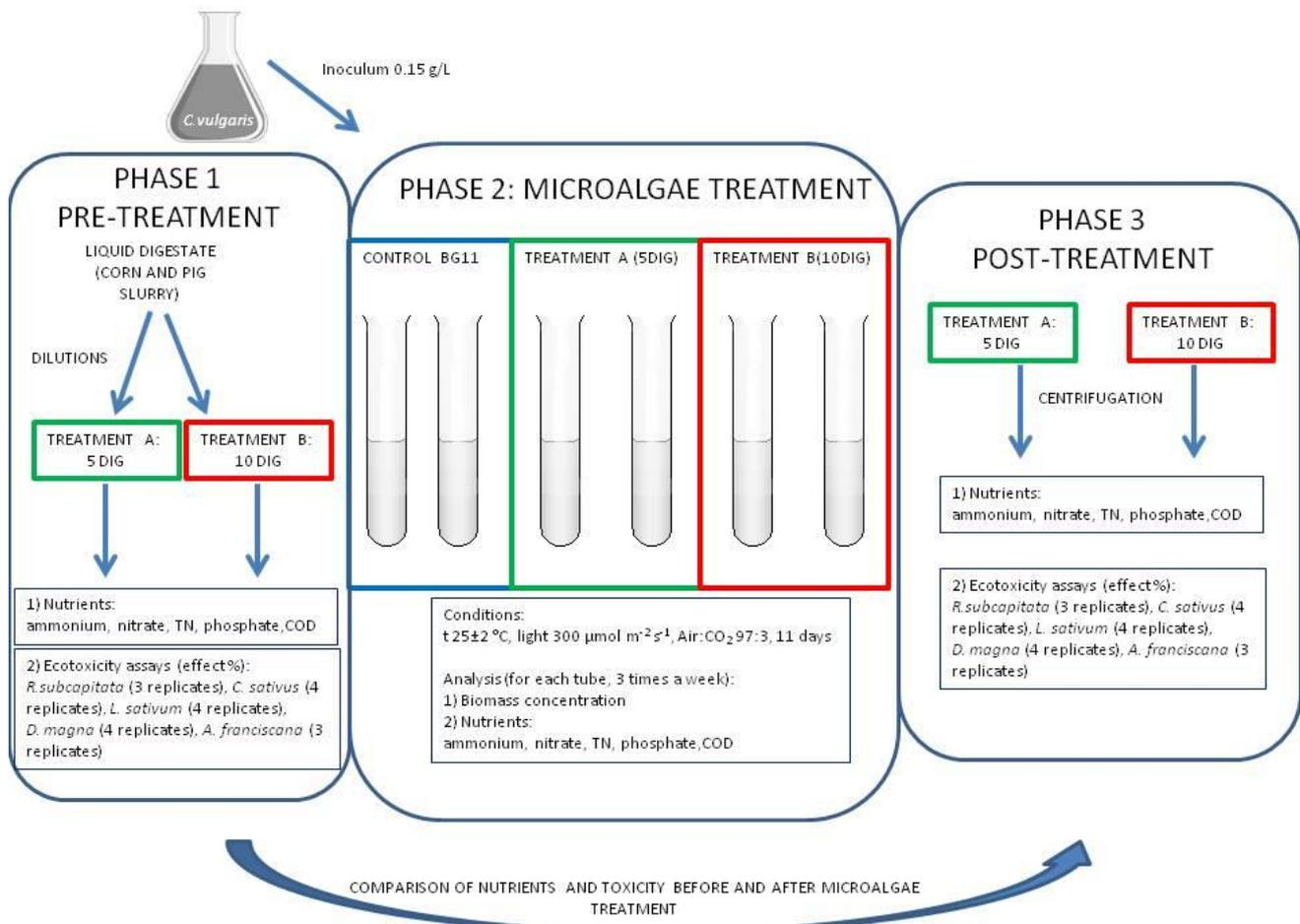
Fig.1 The experimental set-up for evaluating the diluted digestate ( 5% and 10%) treatment with *Chlorella vulgaris*.
