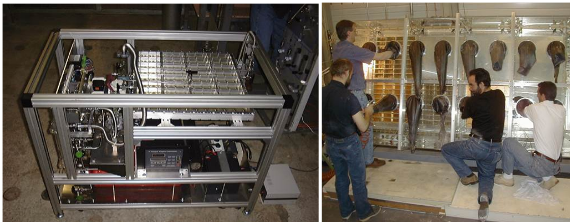
Figure 16. Pictures of the COMPASS photocathode transport system and of the the installation glove-box.
