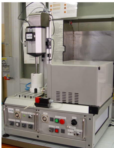
Figure 5. Loop reactor providing MW and US irradiation (Authors' lab)
