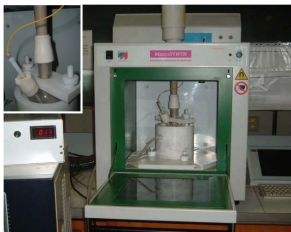
Figure 4. SMUI with a cooling system (Authors' lab)
