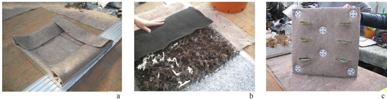
168 Fig. 2. Manufacturing of the final prototype. Fig. 2a) Outer layer of the VGMS (recycled polypropylene). 169 Fig. 2b) Placement of the inner layer (growing medium) of the VGMS. Fig. 2c) Modular box of the VGMS 170 with pockets where the plants were to be inserted.
