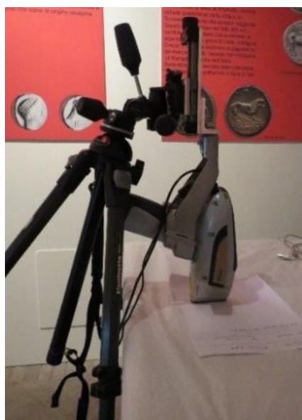
Fig. 2. p-XRF setup during measuring session in museum.
