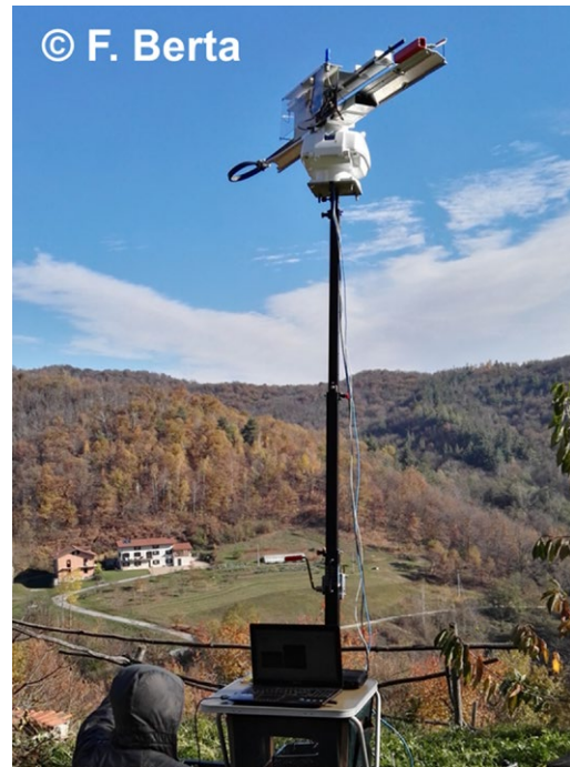
FIGURE 1 New setup of the harmonic radar for the yellow-legged hornet tracking; the radar currently operates on top of a telescopic portable tower which allows to get rid of obstacles shorter than about 6 m
