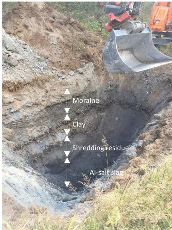
Figure 4: Landfill layers at the Vierumäki industrial landfill.
