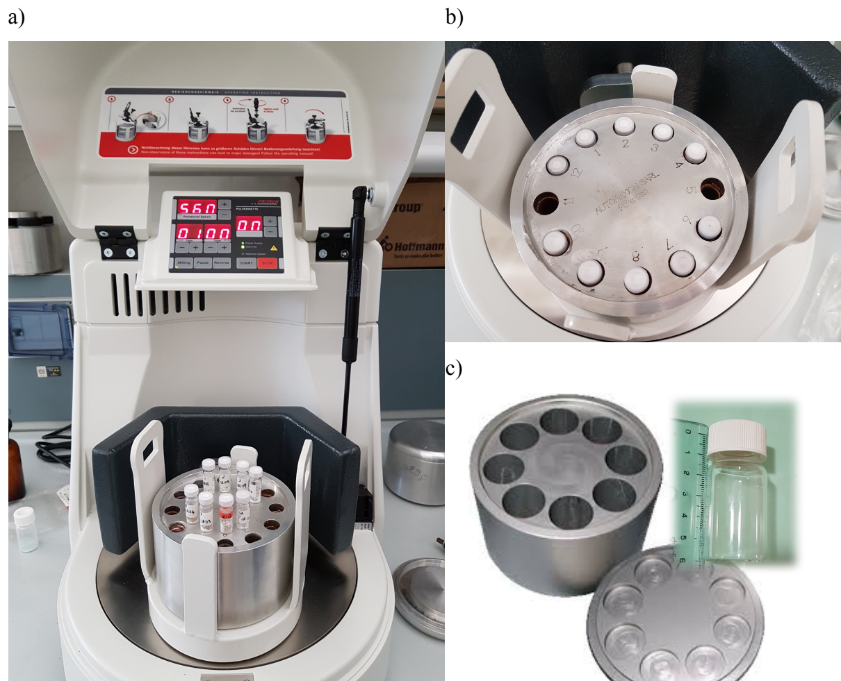
Figure 1. a) A multisampling planetary mill for more details visit http://www.automaxionltd.com/ ; b) 12 position jar hosting 2 mL GC/LC glass vials; c) 8 position jar hosting 20 mL glass vials.
