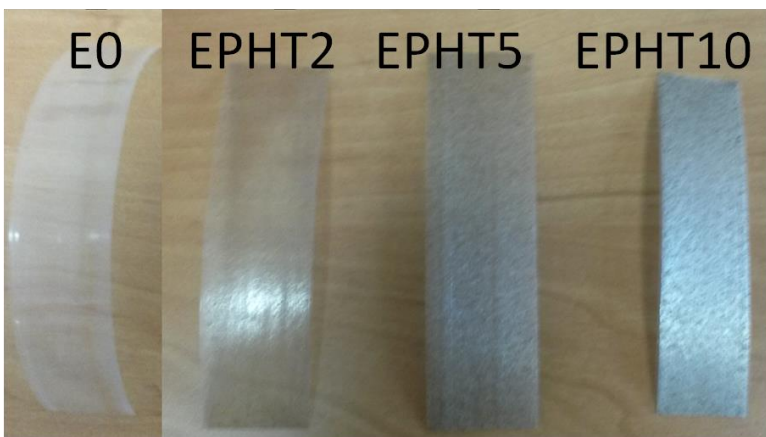
Fig. 2. Blend sheet films at different filler contents. Legends as in Table 3
