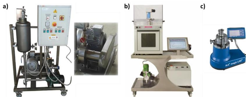
**Figure 1.** a) Rotor-stator generator of hydrodynamic cavitation \_E-PIC S.r.l. (Turin, Italy). b) The configuration of FlowSynth Microwave system (Milestone S.r.l.). c) High-Shear Mixing (Magic-Lab, IKA).
