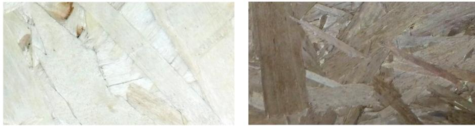
**Figure 1.** Appearance of poplar Oriented Strand Board (OSB) pre- (left) and post-thermal treatment (right).
