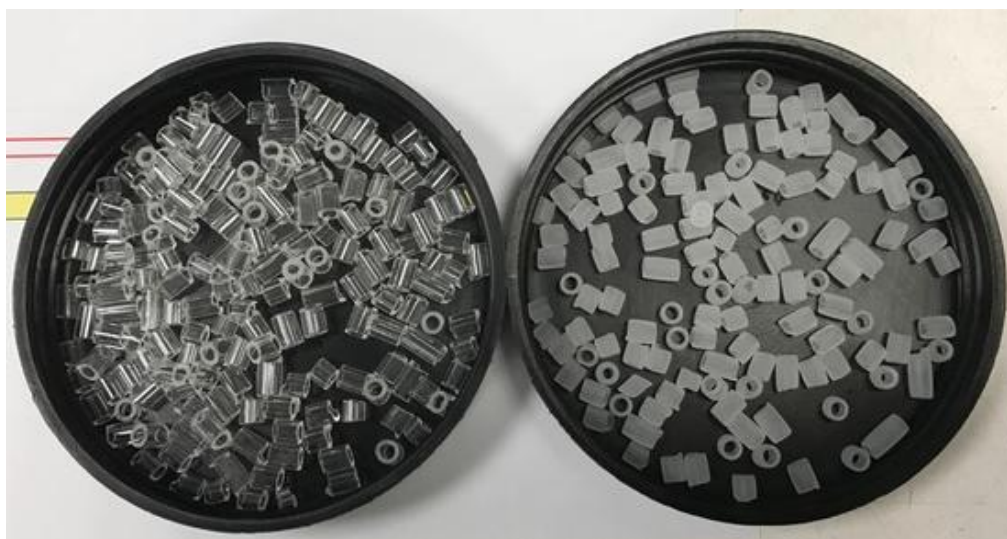
Figure 1: Glass Raschig rings without catalyst (on the left) and coated with a thin film of TiO 2 (on the right).
