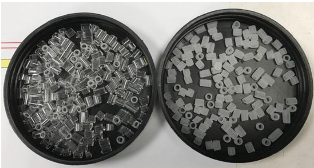
Figure 1: Glass Raschig rings without catalyst (on the left) and coated with a thin film of TiO 2 (on the right).
