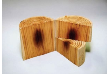
Fig.2: Cross-section of wood after 3 minutes of microwave radiation. Reprinted with permission from M. Miura, H. Kaga, A. Sakurai, T. Kakuchi, K. Takahashi, J. Anal. Appl. Pyrolysis , 2004, 71 , 187–199, Copyright 2018, Elsevier.
