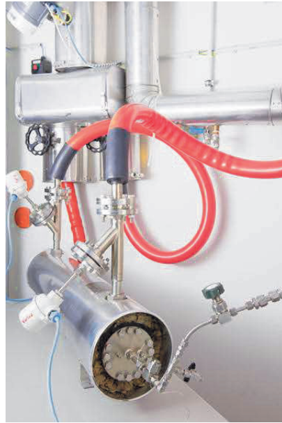
Figure 11: The sodium alanate-based hydrogen storage tank developed during the NESSHY project showing the attachments to the testing rig.
