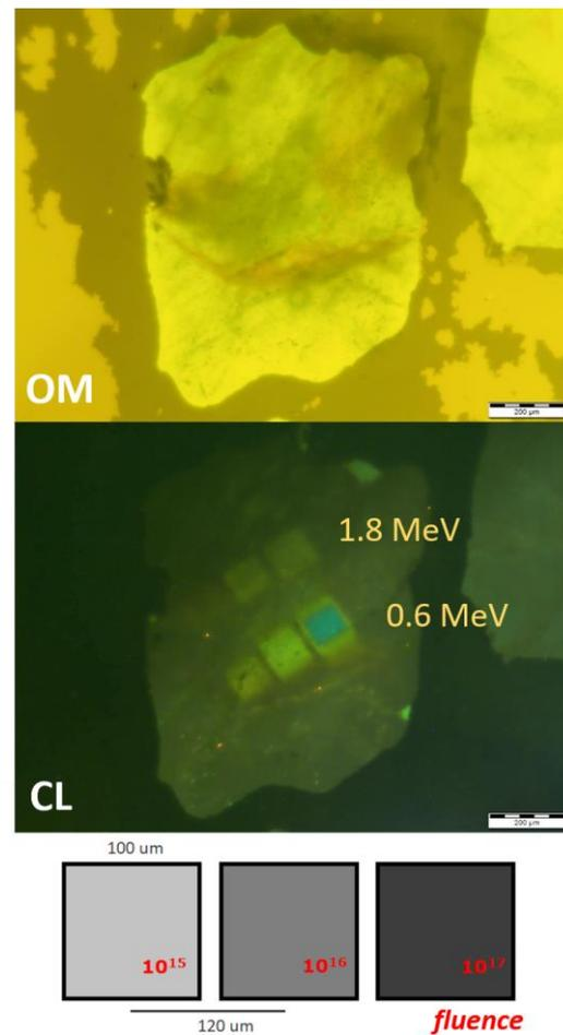
Fig.2 Optical Microscope (above) and cold-CL (below) images of the same quartz crystal from Paung Gu Temple coarse brick; He<sup>+</sup> irradiation was performed in six different areas, with 1.8 MeV (upper row) and 0.6 MeV (lower row) energy combined with three fluence values (10<sup>15</sup>, 10<sup>16</sup> and 10<sup>17</sup> ions/cm<sup>2</sup>). Scale bars are 200  $\mu$ m long. A scheme of the irradiation pattern is also reported.
