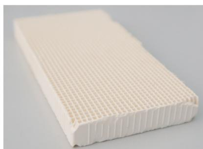
**Figure 6.** The cordierite honeycomb monolith utilized in the photoreactor. Dimensions: 10 × 5 × 1 cm; 1456 channels: 0.17 × 0.17 cm.
