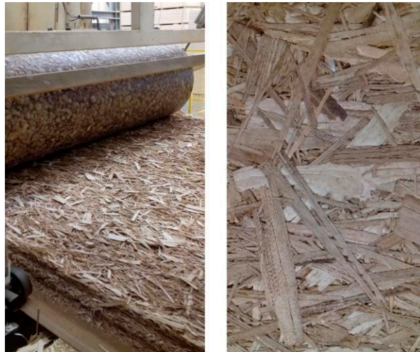
Figure 1. Strand mat before pressing (left) and detail showing the surface of a type B board (40% poplar, 60% sweet chestnut, right).
