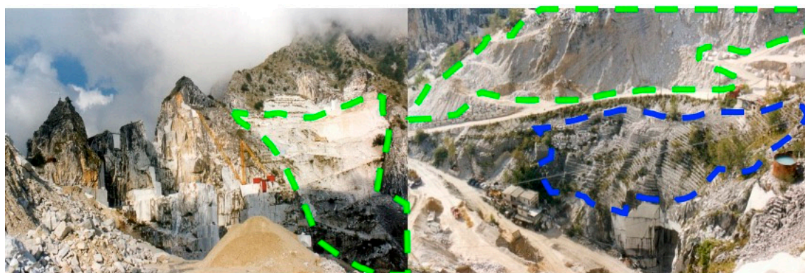
Figure 14. Carrara marble quarrying basin: open pits and Ravaneti (green dashed lines). Some of the historical Ravaneti (blue dashed line) have been used as a base for the internal roads in quarrying areas.
