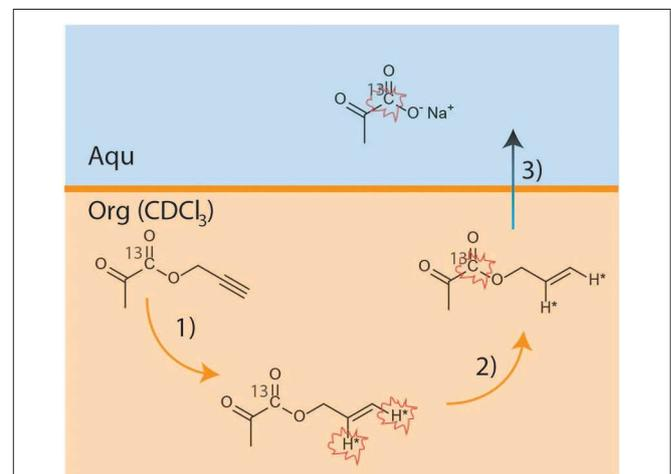
**FIGURE 1** | Scheme reporting the key steps of the PHIP-SAH procedure: (1) hydrogenation using parahydrogen of propargyl- $[1-^{13}\text{C}]$  pyruvate; (2) polarization transfer to the  $^{13}\text{C}$  carboxylate spin by means of magnetic field cycle (MFC); (3) hydrolysis and phase transfer of the Sodium salt from the organic to the water phase.
