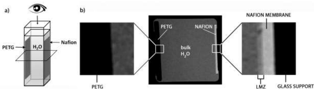
FIGURE 1: a) schematic representation of the phantom used for the acquisition of MR images: PETG and Nafion samples are fixed on the walls of a cuvette filled with water; b)  $T_1$ -weighted image of water protons in the presence of N115 (on the right) and PETG (on the left), axial projection. The LMZ is visible on the Nafion surface but not on PETG.
