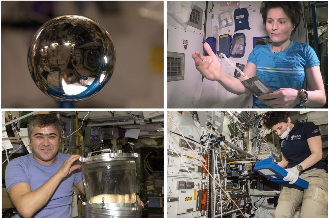
Figure 1. A water drop floating on the ISS (upper left). The Italian astronaut Samantha Cristoforetti and the Russian cosmonaut Salizhan Sharipov showing the Teflon bag (upper right), the water tank (lower left) and removal system (lower right), used for drinking purposes and water storage on the ISS (Credits: ESA and NASA).
