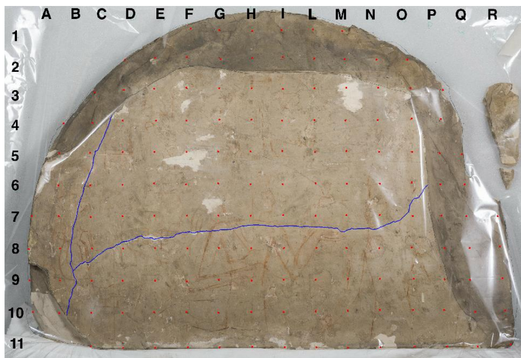
Figure 2. The image shows the dot pattern employed to carry out the ultrasonic test.
