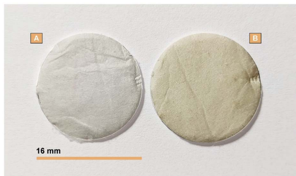
Fig. 6 GLU2_16 spun mat (A) before and (B) after the thermal treatment.
