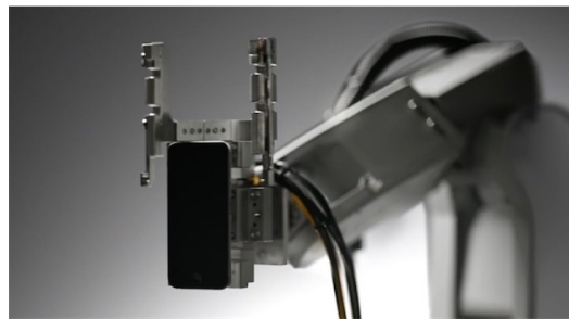
Figure 5. Liam, a collaborative robot by Apple which disassembles iPhones.
