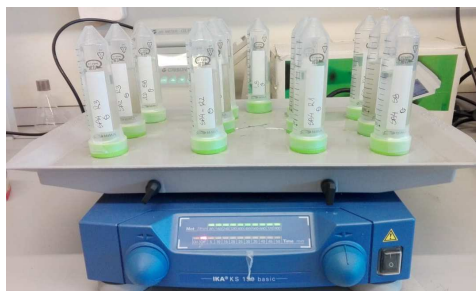
Figure 1. Setup for orbital shaking in liquid sludge LLE method
