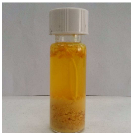
Figure 1. Vial containing the sample with the packed capillary to start the direct extraction.
