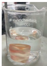
Fig. 1. Cup-shaped 3D printed device with covalently attached antibody for diclofenac extraction.
