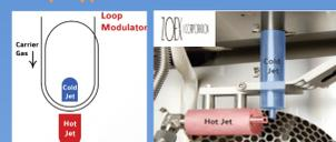
"Single jet - two stage modulator" deactivated silica capillary is rolled up in a loop held by a metallic glide.
