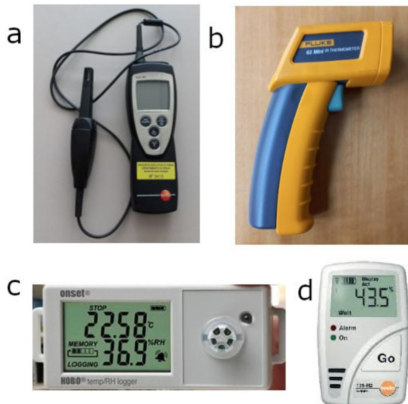
**Figure 3.** Instruments: (a) Testo 625 thermo-hygrometer, (b) Fluke 62 Mini infrared thermometer, (c) HOBO-UX100-011 thermo-hygrometer, and (d) Testo 175-H2 thermo-hygrometer.
