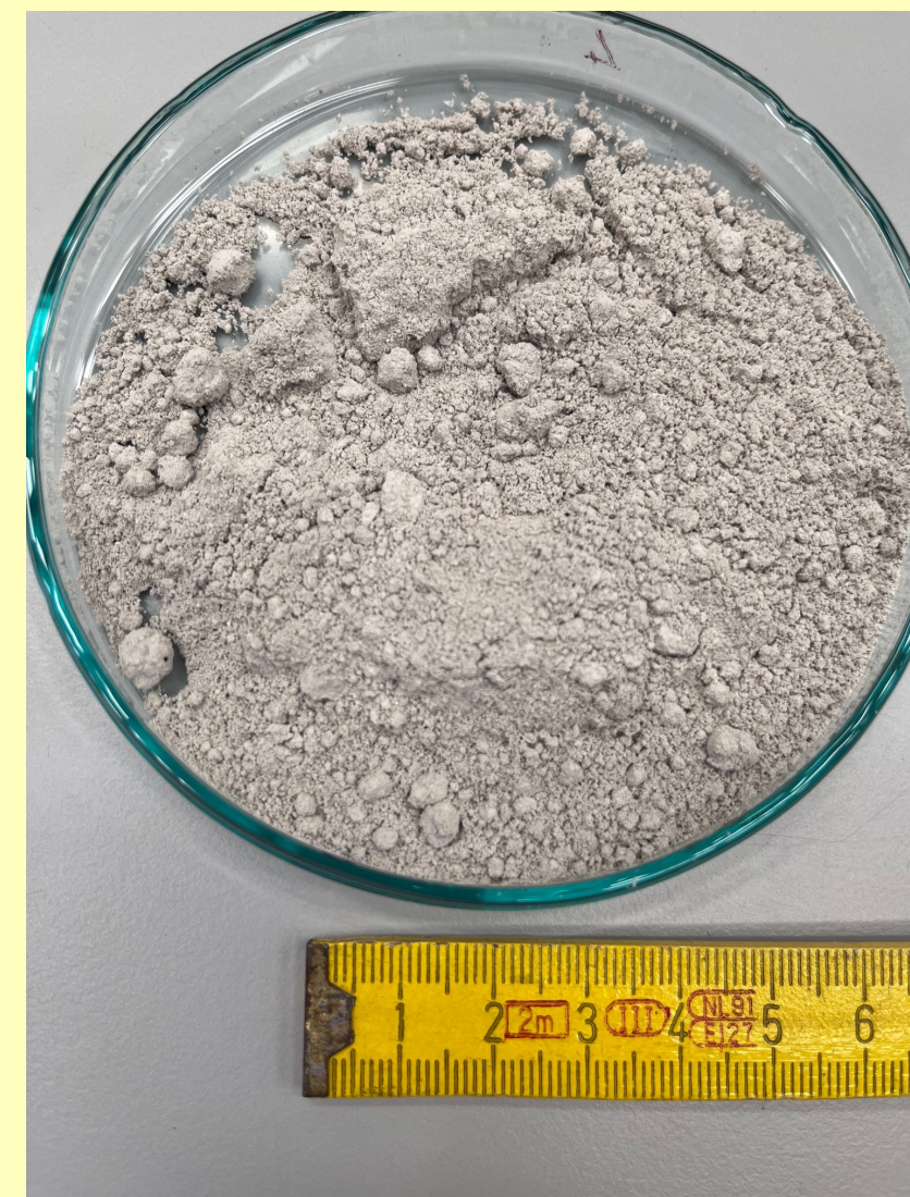
MSWI fly ash raw sample. The particle size is fine and D50 is 149 μ.
