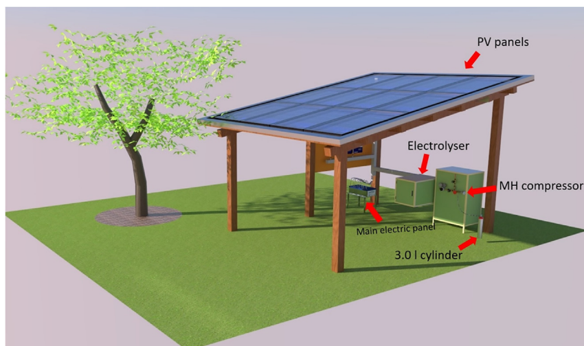
Fig. 1 – Schematic representation of the hydrogen refuelling station.
