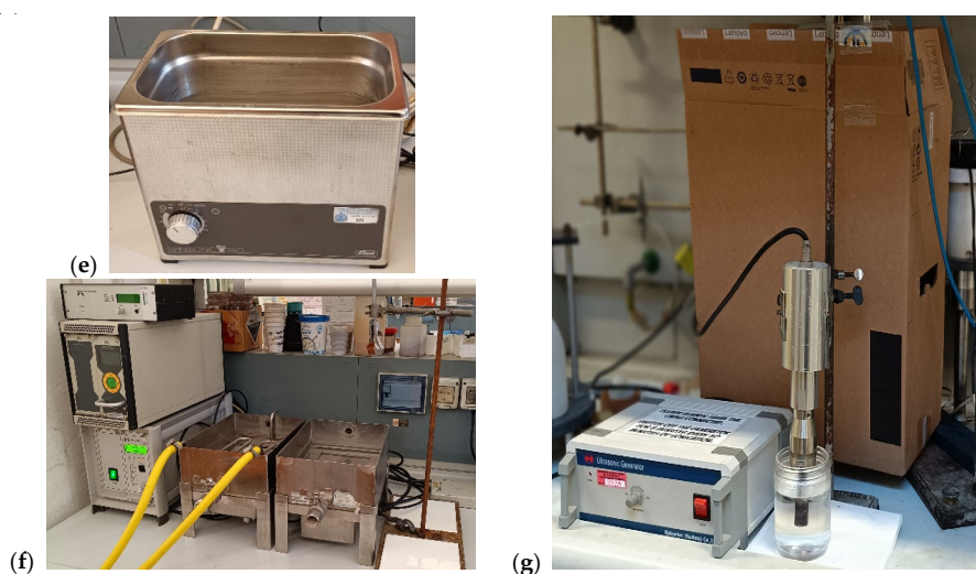
Figure 3. Instruments for cavitation experiments. Pictures of (a) and (d–g) were photographed by the authors. (a) Ultra-turrax; (b) schematic view of simple Venturi tube, Liu and Li [85]; (c) schematic view of Venturi tube with reagent inlet, Tang et al. [86]; (d) laboratory-scale Venturi-instrument; (e) laboratory (cleaning) bath ultrasonicator with single frequency and energy level; (f) laboratory bath sonicator with controllable frequency and energy; (d) horn-type laboratory sonicators with controllable energy level.
