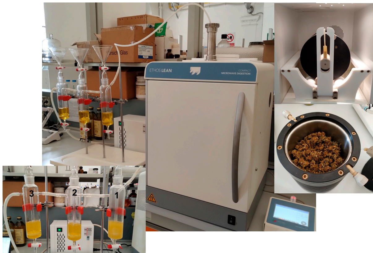
Figure 1. Ethos LEAN MW oven configuration for the capture of Cannabis terpenes in olive oil (Milestone Srl).
