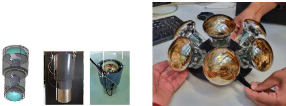
Figure 2. Prototypes of single large PMT (left panel) and of a system of multi PMT composed by seven 3'' PMTs (right panel).
