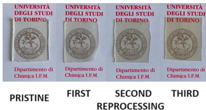
Figure 6. Comparison between the pristine network (first image) and the first, second, and third reprocessing (following images).
