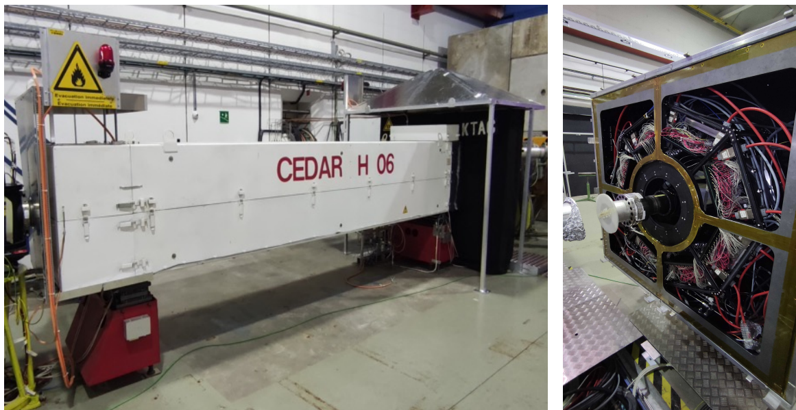
Figure 9. CEDAR-H (left panel) and KTAG photon-detection system (right panel) during installation in the experimental hall. In the left panel, the downstream end of CEDAR-H is on the left, and the black enclosure of the KTAG photon-detection system is on the right. In the right panel, the upstream-side of the enclosure is removed, revealing the eight sectors within.
