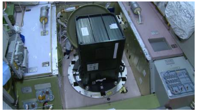
Fig. A.1. Mini-EUSO detector installed inside the ISS on the UV transparent window of the Zvezda module. The round porthole on the bottom of the picture looks nadir; the bottom centre part (marked '1') is oriented toward the direction of the velocity vector of the station (Bacholle et al. 2021).
