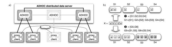
Figure 1. a) Typical architectural schema of applications based on ADHOC. b) Example of two different distribution and replication schemas (**①** and **②**) for a collection K of objects a, b, c, d over 4 ADHOC servers S1, S2, S3, S4 (grey objects are replicas).
