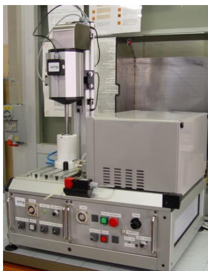
Figure 1. Commercially available system for sequential US/MW irradiation (NTS - Vicenza).
